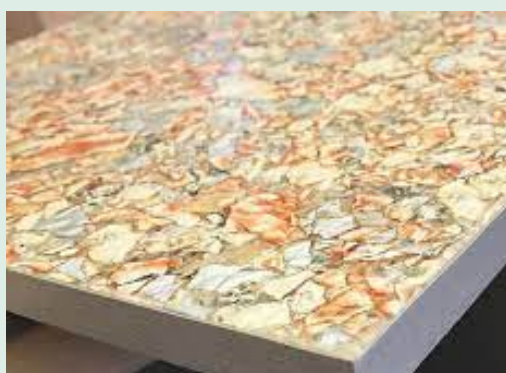
Walls made from recycled beverage cartons
